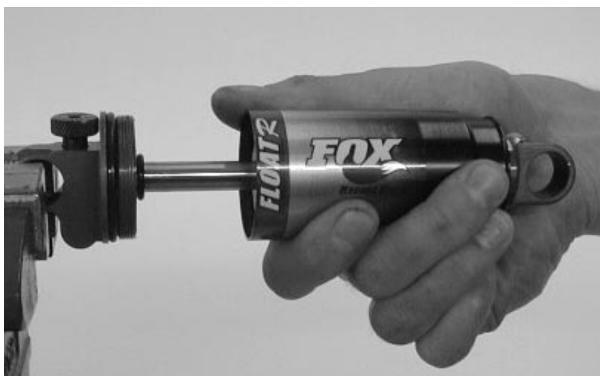
Figure C. Air Sleeve Installation.
