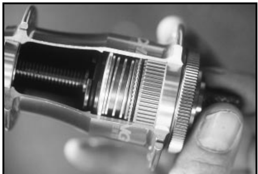
Figure 22 - capture whole RingDrive™ assembly
