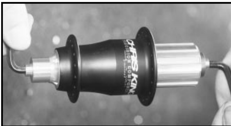
Figure 11 - disassemble main axle
