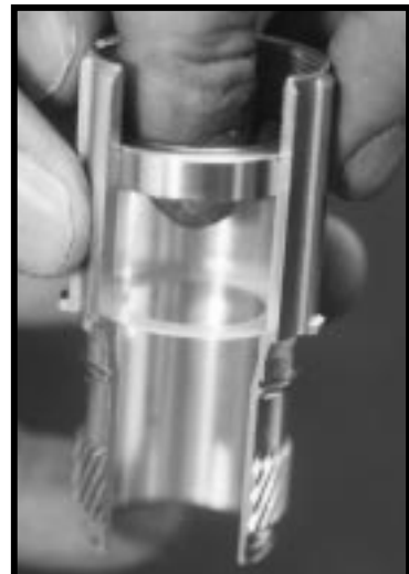
Figure 34 - drive shell seal & bearing
