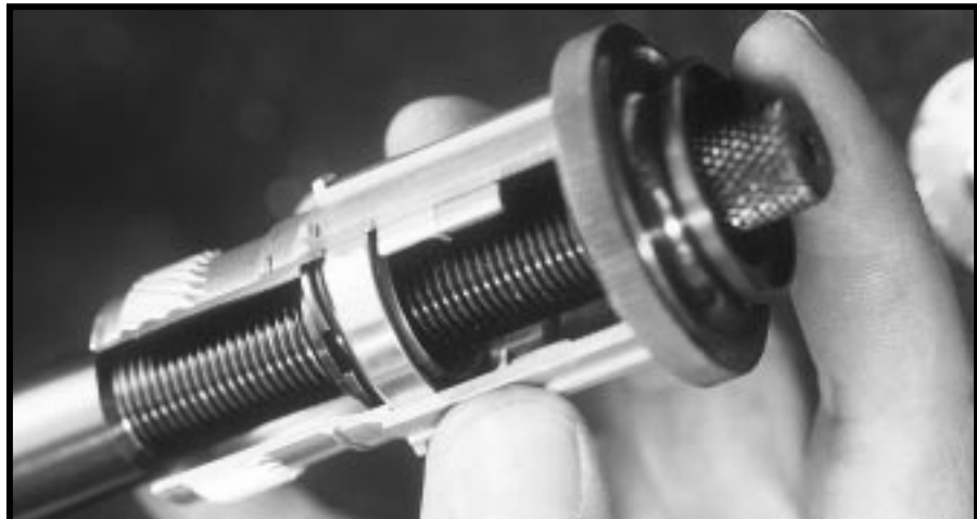
Figure 24 - remove drive shell bearing
