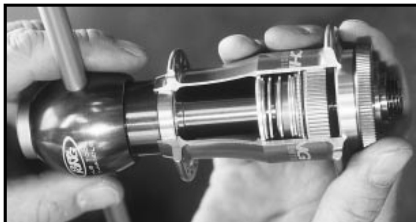
Figure 33 - press drive side bearing
