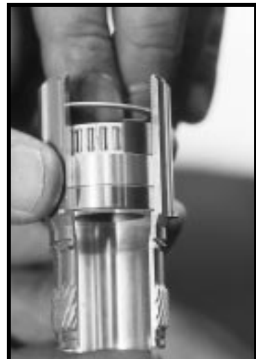
Figure 36 - needle bearing & capture plate
